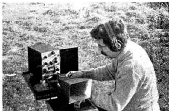
—here is F2FO at the receiving end, copying the 'RPE signals. This receiver employed a balanced mixer in conjunction with a 2K25 klystron oscillator to provide an i.f. which was 5MHz wide at 50 MKz, starting off with a low noise 417A cascade followed by five 6AK5 stages. The horn aerials included in these illustrations produced a gain of 24dB.
